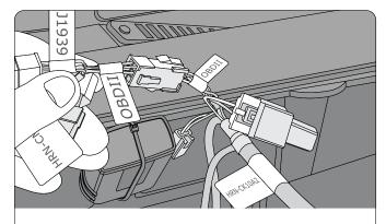
Step 6B: Connect the OBD II-labelled 6-pin white Molex connector from the HRN-CK10A2 harness to the OBD II-labelled 6-pin white Molex connector from the HRN-CM24Y1 harness.
