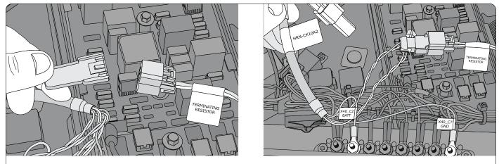
Step 4B: Locate the 2-pin J1939 connector in the fuse box and remove the EOL resistor.
