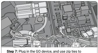
ep 7: Plug in the GO device, and use zip ties to secure the device and harnesses.
